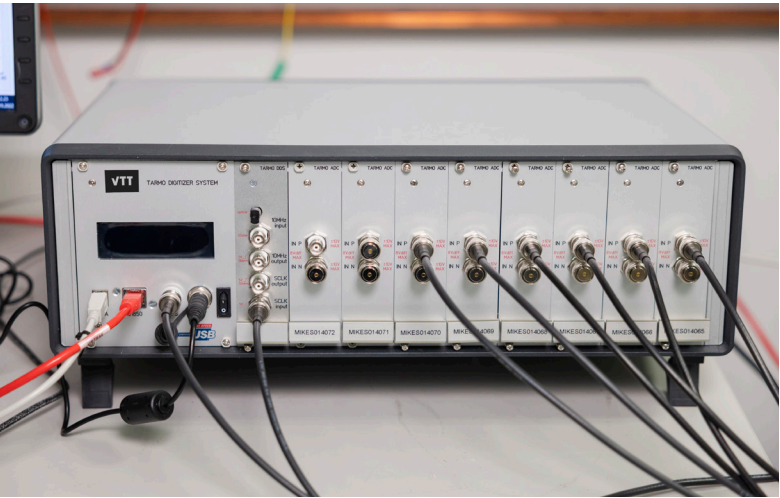
VTT Tarmo used as a sampling AC measurement standard. A separate scaling device can be used for extending the input range.
